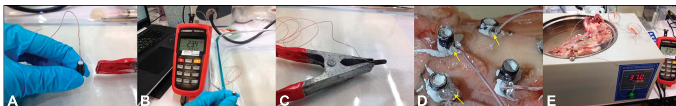
Fig. 1. (A–E) The hollow space of the implant was filled with thermal paste, and the tip of a thermocouple was inserted into that space. (A) The other end of the thermocouple was connected to a temperature logger. (B) The cap end of the thermocouple was held with a clip and covered with an electrical tape to prevent the mist from getting to the thermocouple. The body of the implant was left exposed and available to be irradiated with the laser. (C) Holes were drilled into the pig jaw using the SOLEA laser and filled with thermal paste. Each implant was placed into a hole, and the tip of a thermocouple was situated in the space between the tissue and the thermocouple. A second adhesive covered was used to protect the thermocouple from the mist. (D) The pig jaw was placed in a 37°C water bath (yellow arrows) (E).
